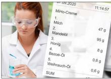
Clear printout with date and time. In addition, the components of the mixture are numbered automatically and printed out with the name and weight
