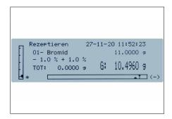
Convenient recipe-weighing: with the recipe database, up to 99 recipes can be stored, each with up to 20 recipe ingredients with name and target value
