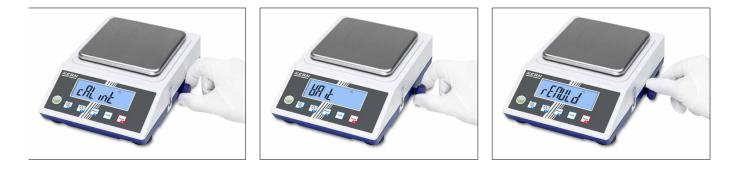
Internal adjustment using the rotary control on the side guarantees a high degree of accuracy and means it can be used in any location
